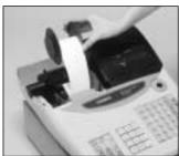
Step 9 Place the take-up reel into place behind the printer, above the roll paper.
