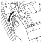
**3** Note the (+) and (–) markings in the battery compartment. Load a set of two new "AA" type alkaline batteries so that their plus (+) and minus (–) ends are facing as indicated by the markings.
